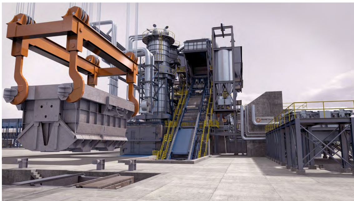
Computer animated 3D image of EAF Quantum electric arc furnace by Primetals Technologies
