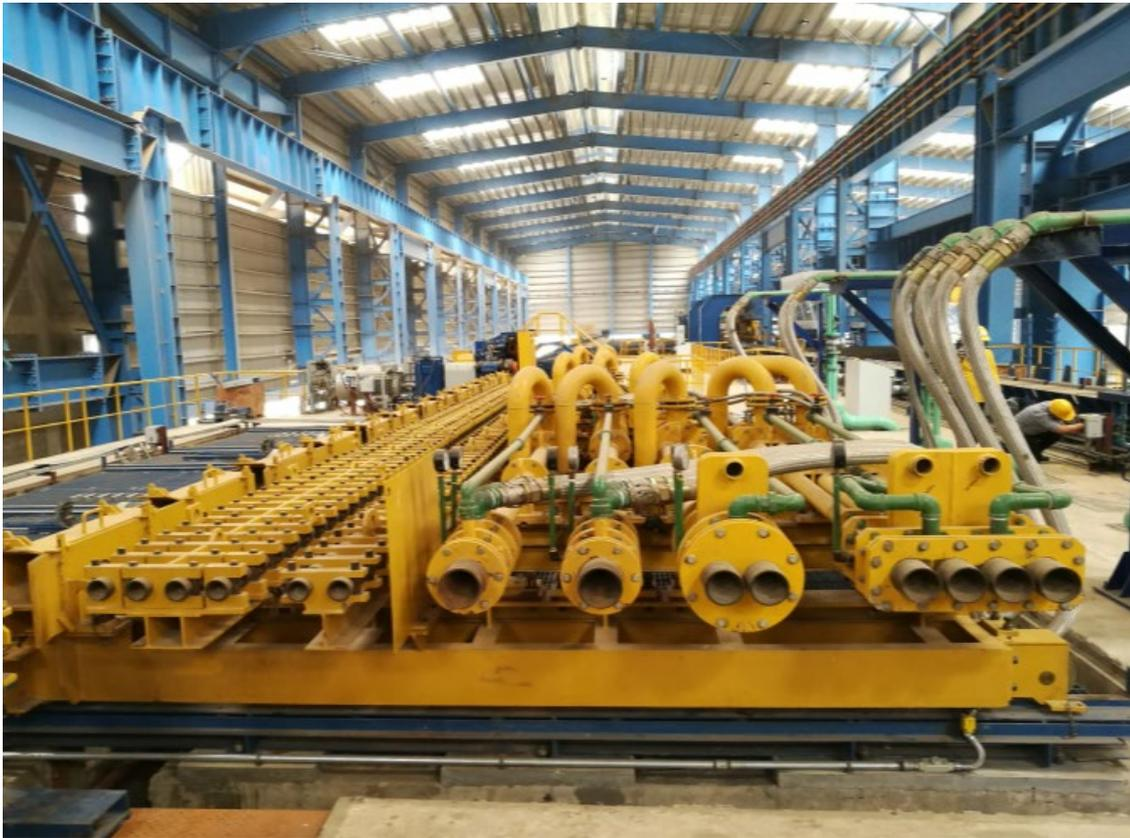
The inline PQS quenching system from Primetals Technologies gives bars a tempered martensitic case and a ferritic-pearlitic core. The PQS is part of Primetals Technologies' supply of a continuous billet caster and a rebar rolling mill for the mini mill project of Naveena Steel in Pakistan.
