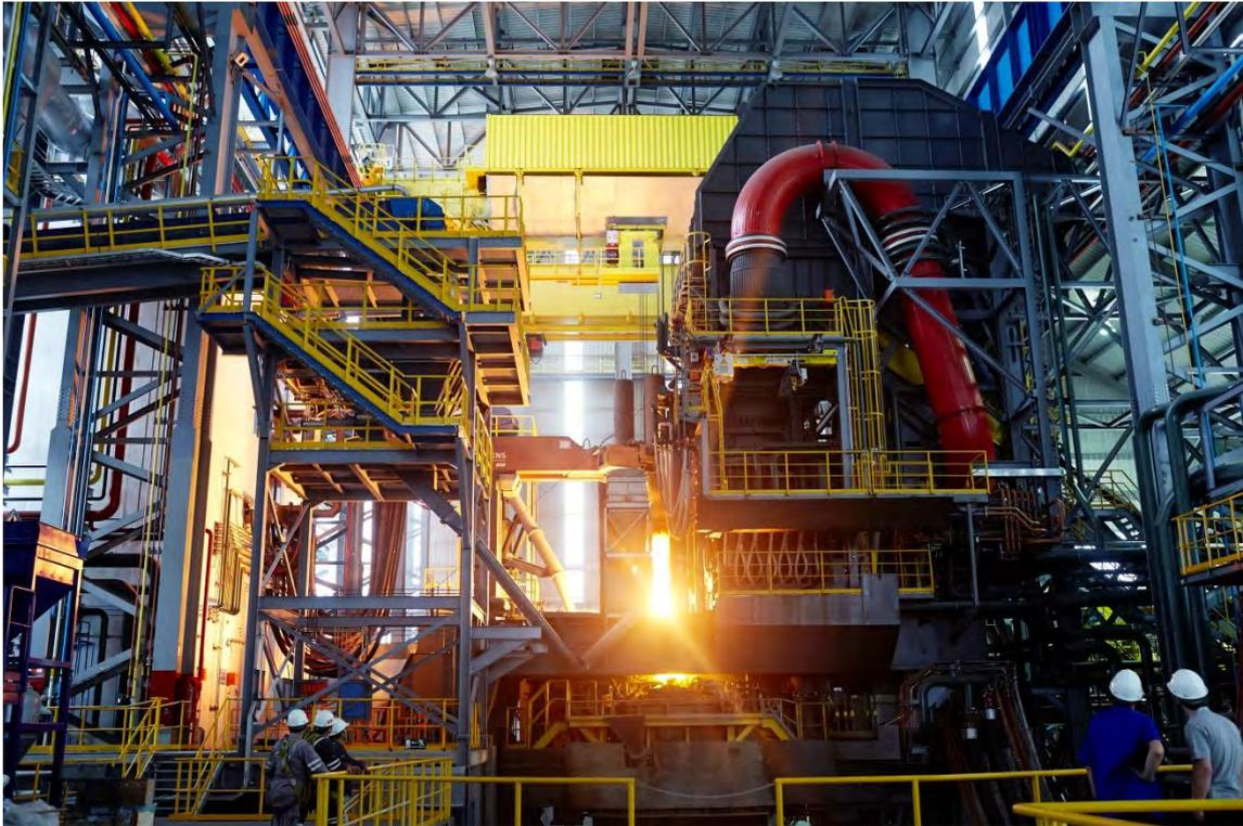
EAF Quantum electric arc furnace from Primetals Technologies
