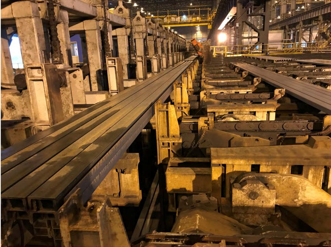
Stacking station for sections from Primetals Technologies
