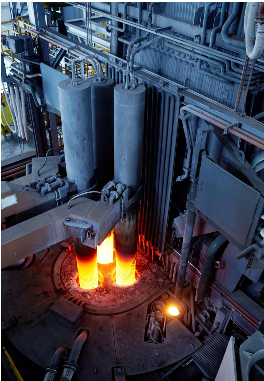
EAF Quantum electric arc furnace from Primetals Technologies
