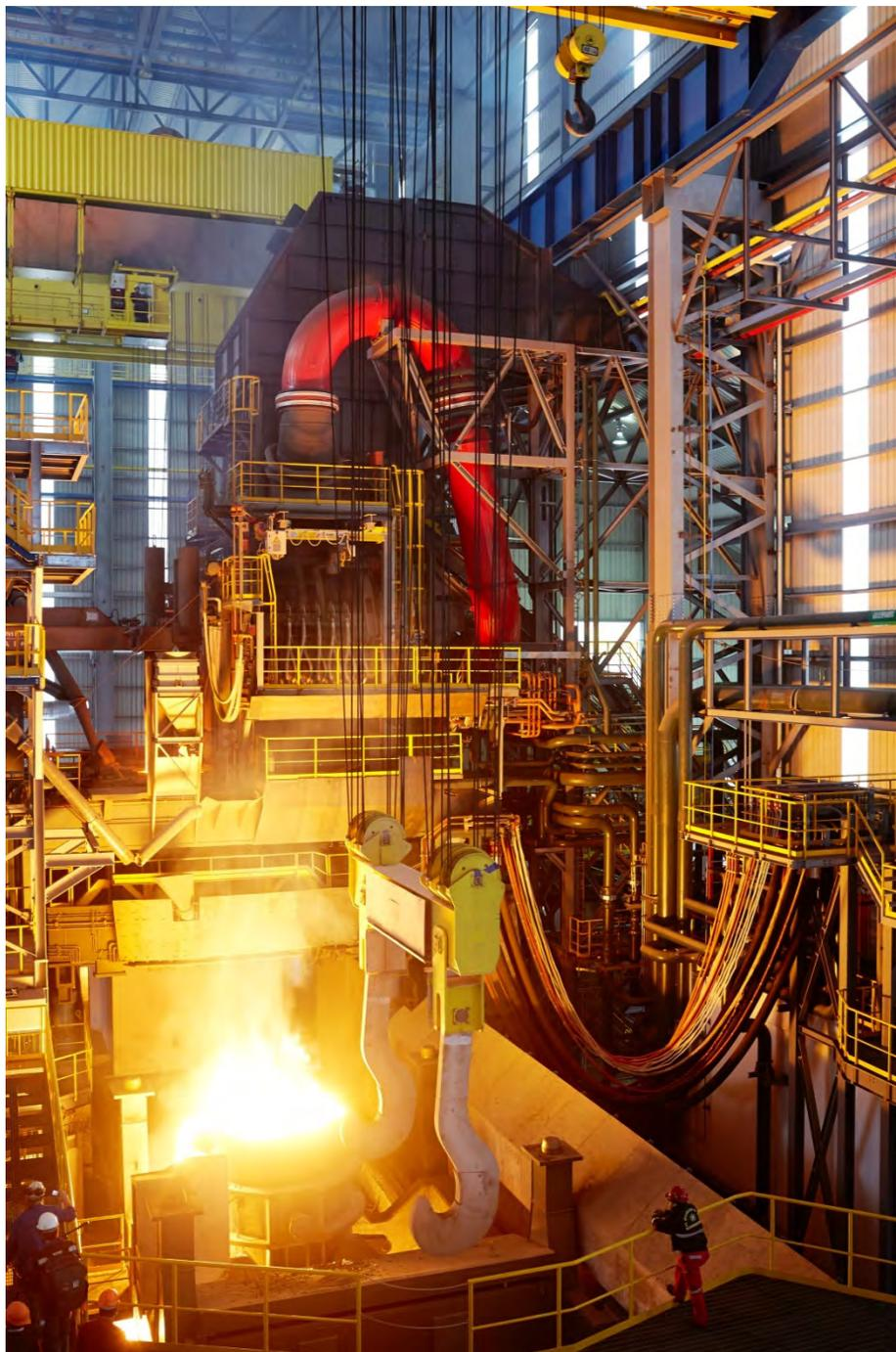
EAF Quantum electric arc furnace from Primetals Technologies
