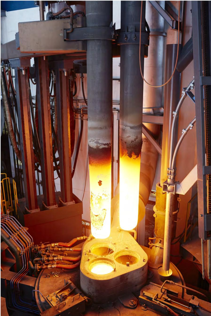
Ladle heating station from Primetals Technologies.
