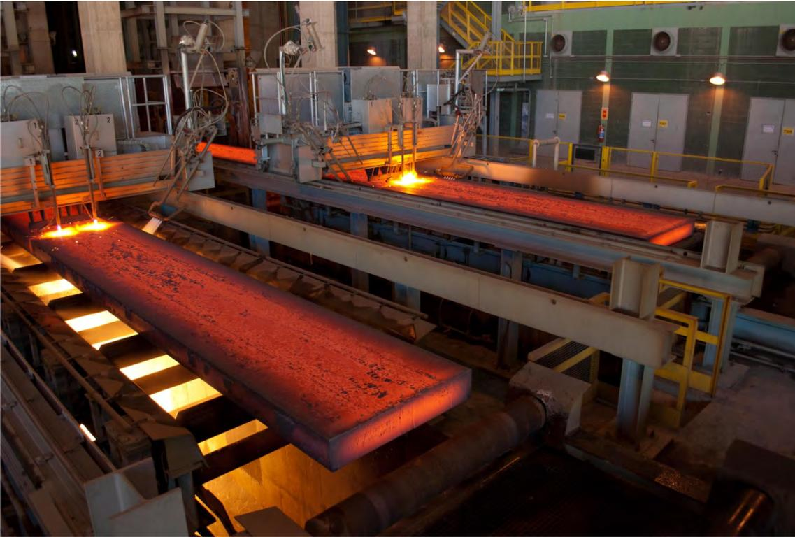
Example of a continuous slab caster from Primetals Technologies. A similar caster will be installed in the Dolvi plant of JSW Steel in India.
