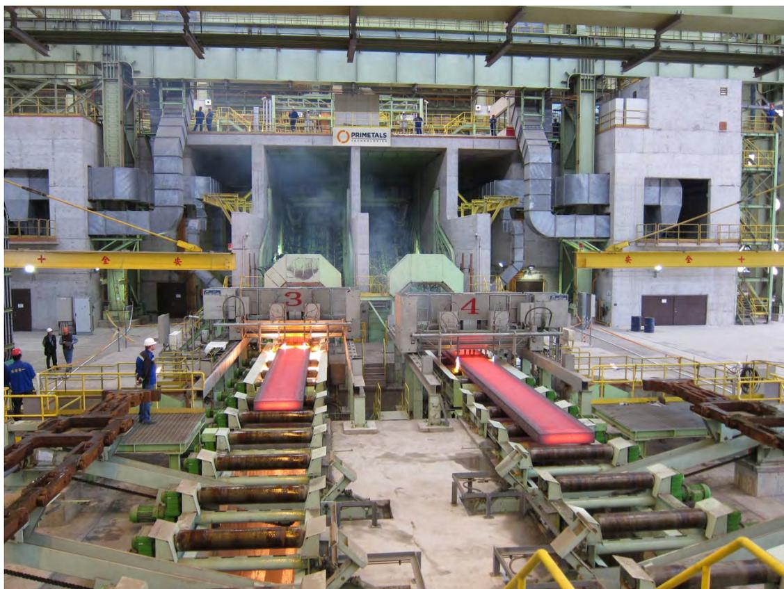
Twin-strand continuous slab caster from Primetals Technologies
