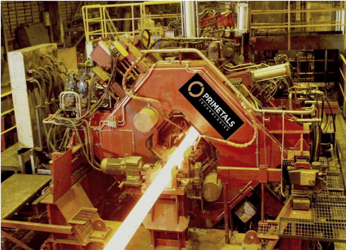
ERT-EBROS billet welding system from Primetals Technologies. A similar system will be installed at Ferriera Valsabbia S.p.A. in Odolo, Italy.
