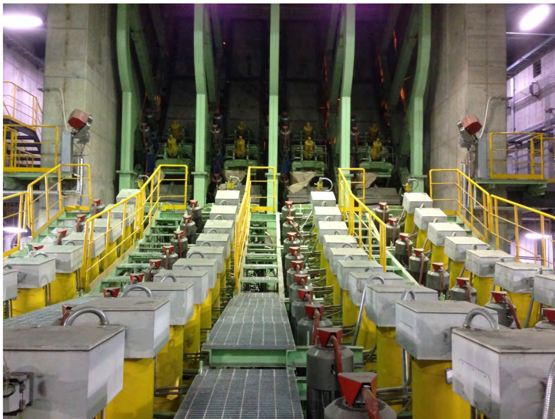
Continuous bloom caster from Primetals Technologies at Hyundai Steel in Dangjin, Korea
